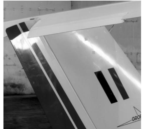
**Fig 5-8** The 'T' tail Plane
