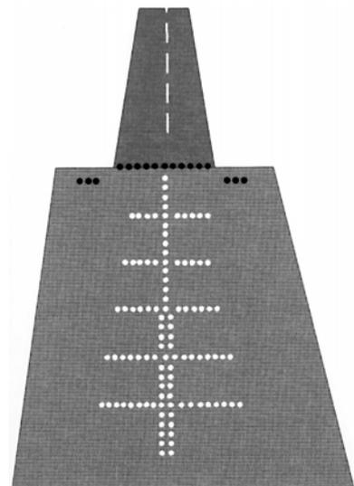
This pattern helps the pilot to judge the aircraft's height and to line up with the runway on the approach to land. In addition, these high-intensity white lights are invaluable in conditions of poor visibility by day, as well as at night, in helping the pilot to find the approach path visually, towards the end of a radio or radar-controlled approach.
