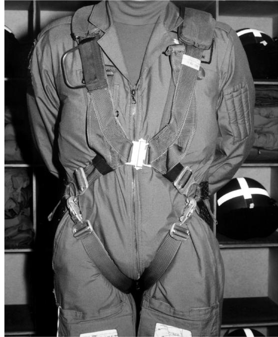
9. Adjustment. There are four adjusters on the harness to allow for different body sizes but the majority of adjustment is done by lengthening or shortening the leg straps.
