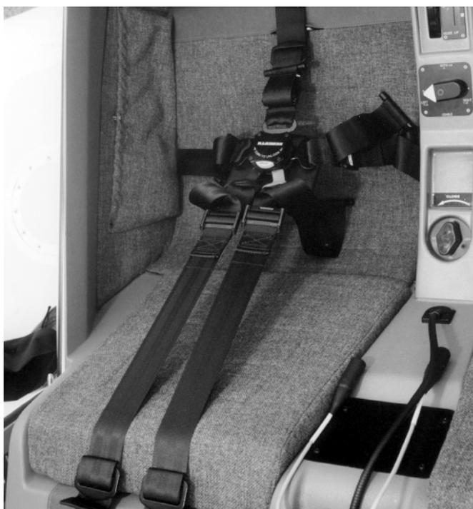
14. Fitting. To fit the aircraft safety harness, loosen off the adjustable straps and insert the four adjustable harness lugs.
