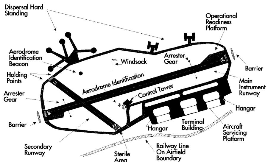
At a typical RAF airfield, the main instrument runway will normally be 45m wide and 1,800m or more long, with subsidiary runways of the same width, but not necessarily as long. At airfields where transport aircraft operate, the main runway is normally 60m wide and 2,700m or more long.
