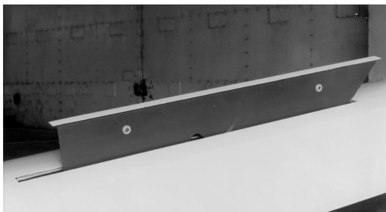
**Fig 4-2** Airbrakes
