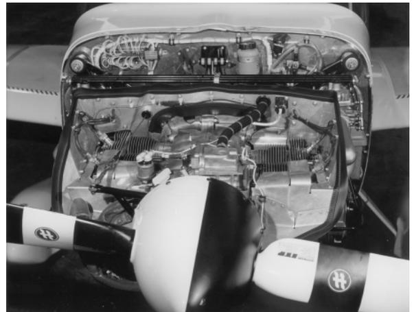
5. GROB 2500 E1 Engine. Power is provided by a GROB 2500 E1 horizontally-opposed 4-cylinder air-cooled petrol engine, developing 95 BHP at 3400 rpm.
